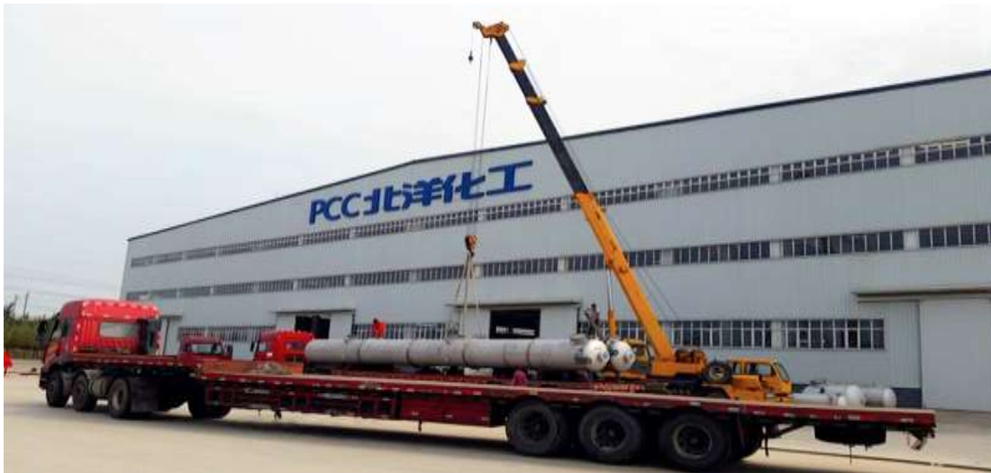
Shangdong Kunda Pyridine refining project Φ1300*48000mm
