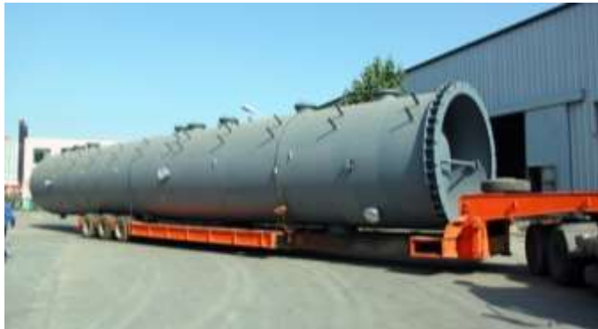
Henan Kaiyuan Air Separation Group Co., Ltd. Jilin Xinda Project Air cooling tower with \Phi 2800\text{mm}
