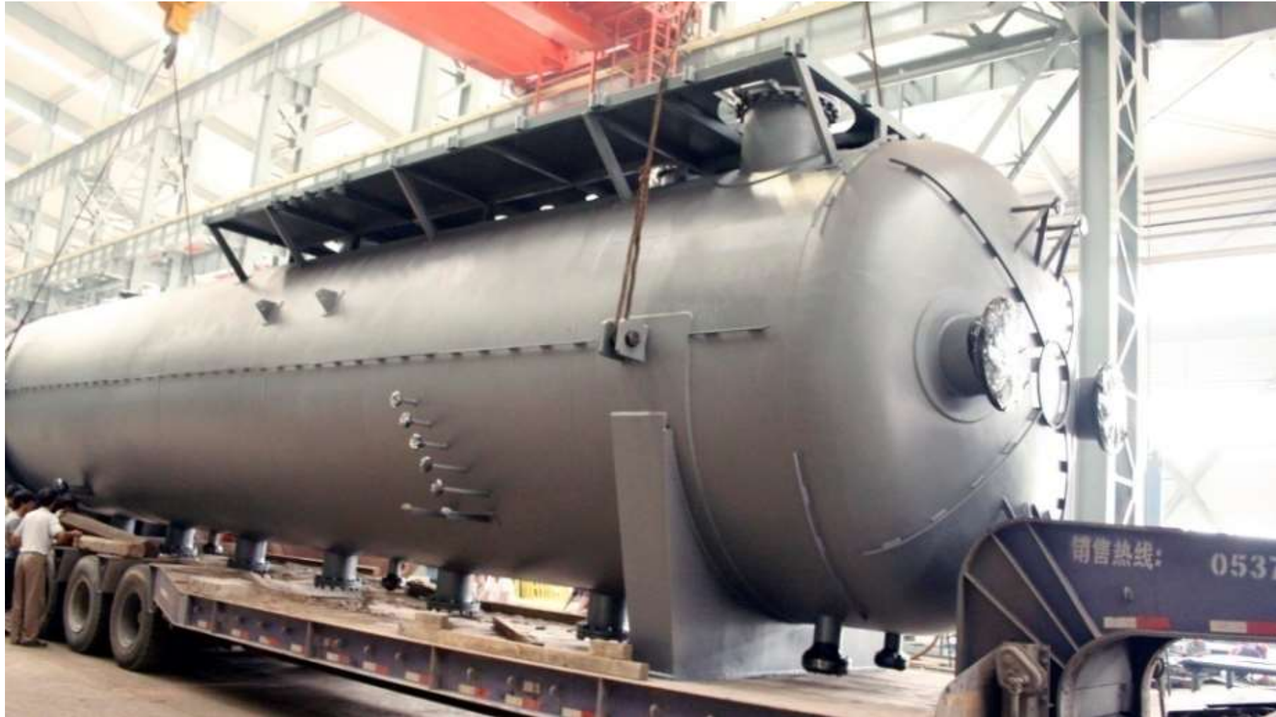
China Oil HBP Group Oil and gas water sand separator \Phi 3000 \times \delta 14000 \times L12
