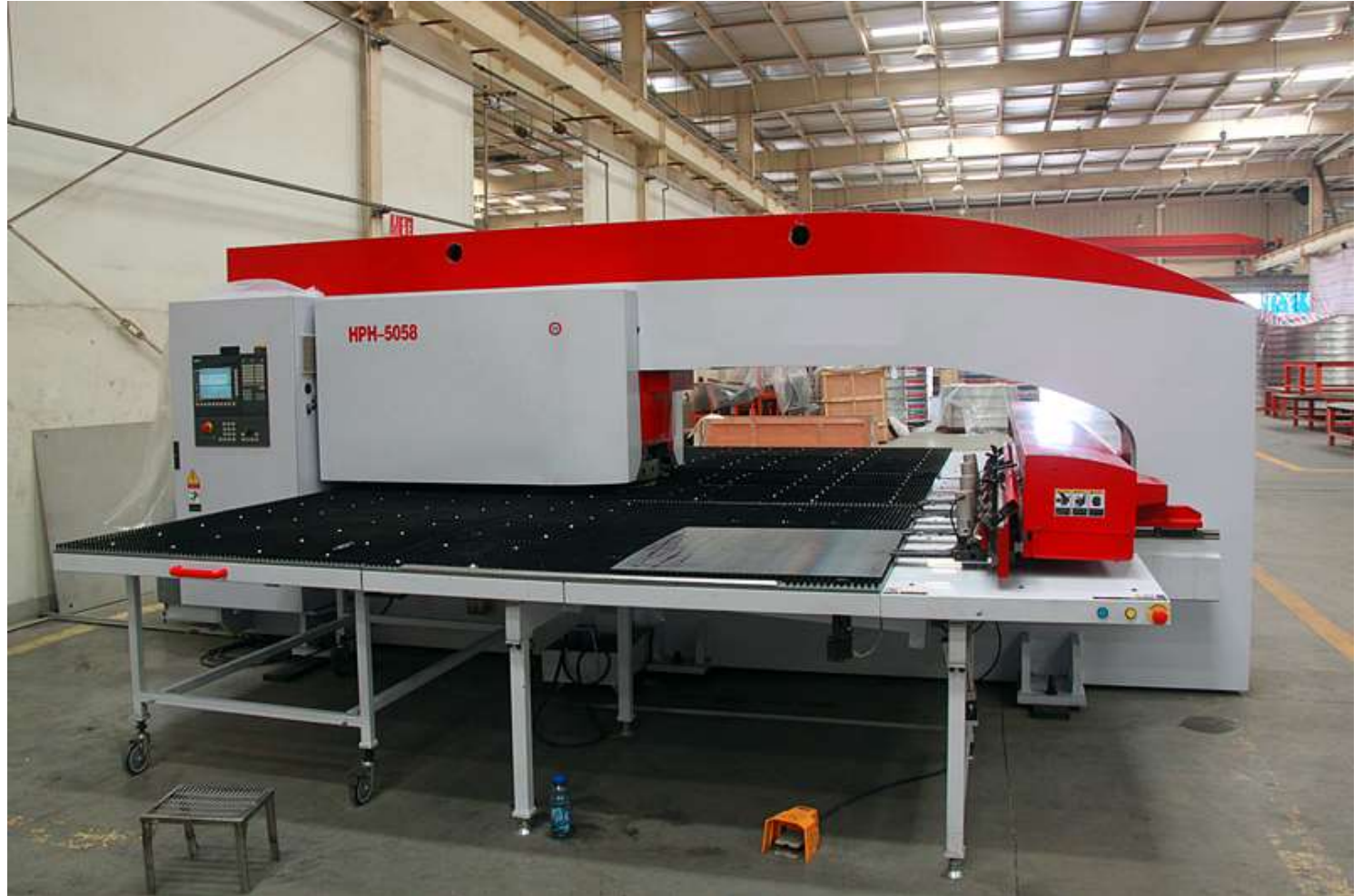
NC turret high speed punch press Used for SS material punching
